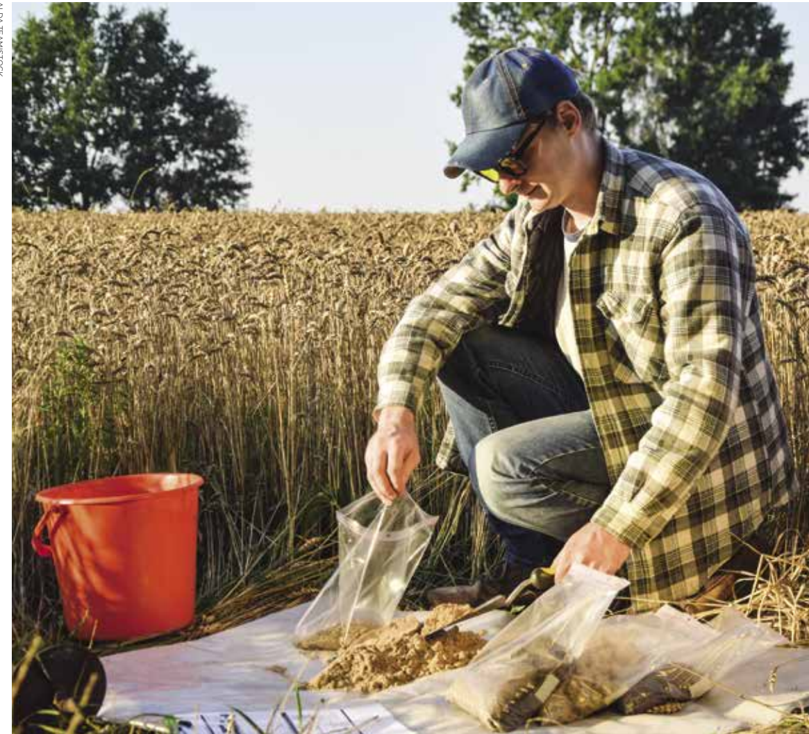
Filling sample bags for laboratory analysis. Remember to accurately map and mark your testing sites!
